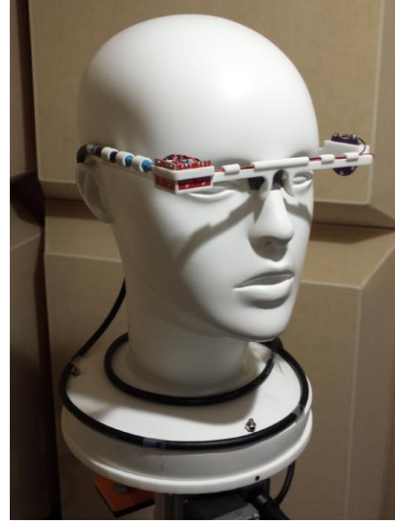
Figure 3: Wearable sound localization prototype, placed on the dummy head.
